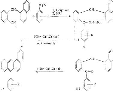
A new and more convenient method has been found for obtaining the 1-(2-cyanobenzyl)-naphthalene (I) required in the synthesis. Bradsher<sup>4</sup> began with crude 2-chlorophenyl- 1-naphthylcarbinol prepared by the Grignard reaction and reduced this
